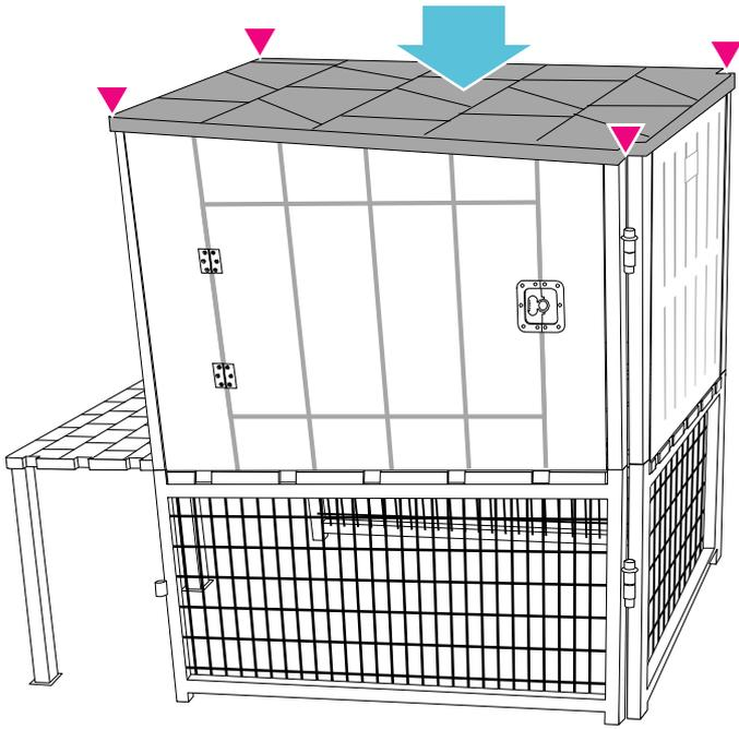
Put the K section which is the footing for your pet to be able to climb the kennel. Install the bolts in the two holes provided for the handle.
