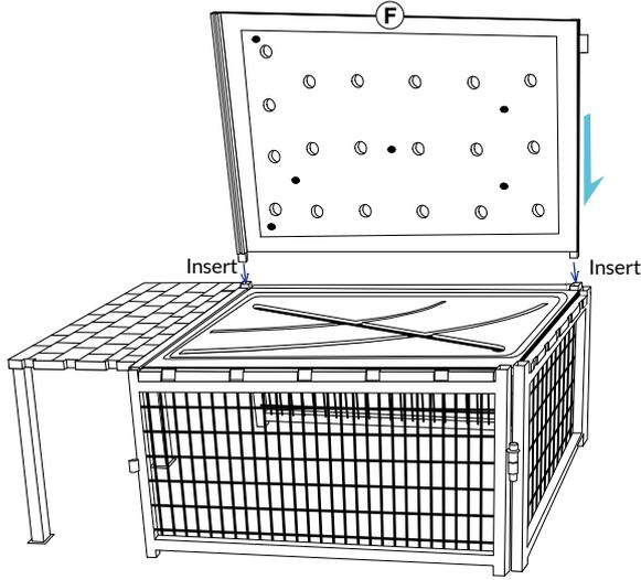
Do the same for the G section, then insert the metal hinge center into the round cavity that meets between F and G.
