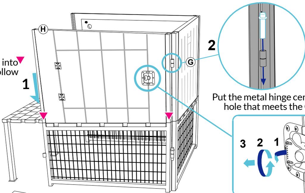
Put the metal hinge center in the hinge hole that meets the G hinge hole.
