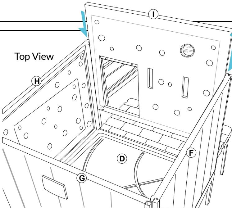
Position the I section into the holder on part H and F, push it down until it touches the bottom. Install the bolts and nuts according to their size.
