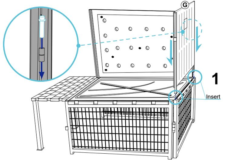
Insert the H leg into the available hollow of part C
